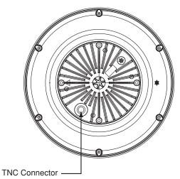
*Figure 3 Antenna Mounting Holes Layout*
