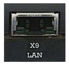
The transceiver has one 10baseT Ethernet port for LAN use.
