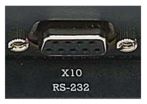
The transceiver has one RS-232 port. The RS-232 port is a standard 9 - pin serial ports with a maximum port speed of 115.2 kbps. It can be used for the following applications:
