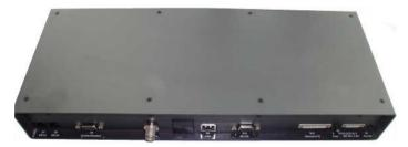
NOTE: It is very important that the unit is placed in an area where access to the hull or equivalent grounding can be reached within 0.5 m.
