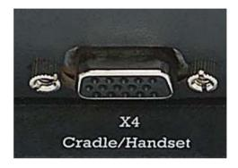
The transceiver has one 4-wire Cradle/Handset ports with RS-485 data control. The handset can be used to setup the terminal and also can be used to make or receive phone calls. The connector outline and pin assignments are described in the figure and table below.
