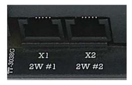
The transceiver has two RJ11 ports, which can be used for connection of analogue phone or fax.
