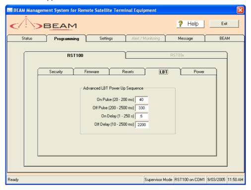
This tab exists to reprogram the power-up profile of a particular LBT if it should end up outside the defaults. It should not be modified from defaults without instruction from technical support.
