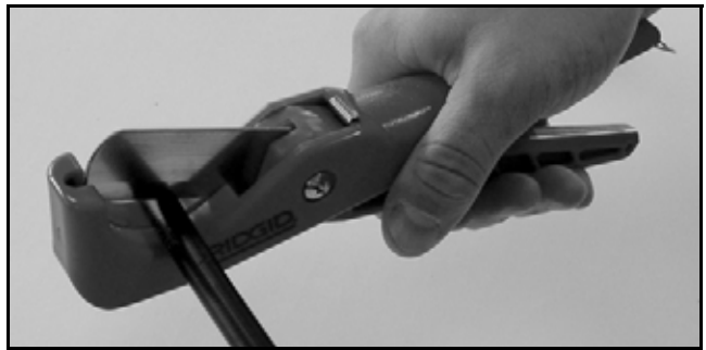
Figure 50: Cutting the Cable
