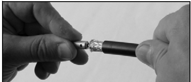
Figure 57: Deburring the Center Conductor
