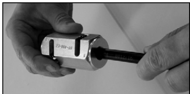
Figure 53: Stripping the End to Expose the Center Conductor
