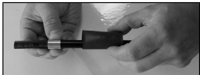
Figure 52: Placing the Heat Shrink Tubing and Ferrule
