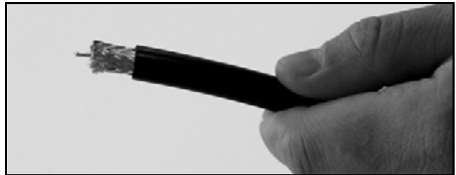
Figure 56: Cable Stripped, Exposing Dielectric
