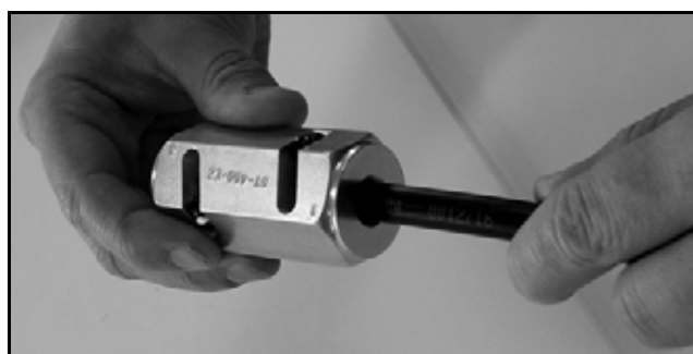
Figure 53: Stripping the End to Expose the Center Conductor
