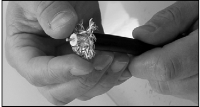
Figure 58: Flaring the Braid
