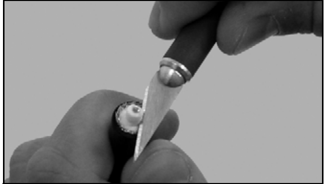
Figure 54: Removing Plastic Residue
