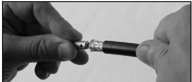
Figure 57: Deburring the Center Conductor
