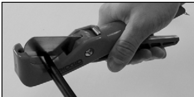
Figure 50: Cutting the Cable
