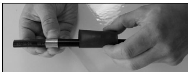
Figure 52: Placing the Heat Shrink Tubing and Ferrule
