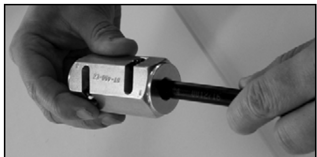
Figure 55: Stripping the End to Expose the Center Conductor
