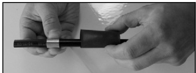
Figure 54: Placing the Heat Shrink Tubing and Ferrule
