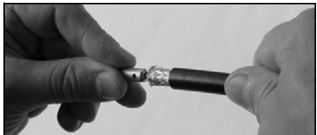
Figure 59: Deburring the Center Conductor
