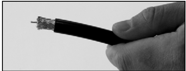
Figure 58: Cable Stripped, Exposing Dielectric
